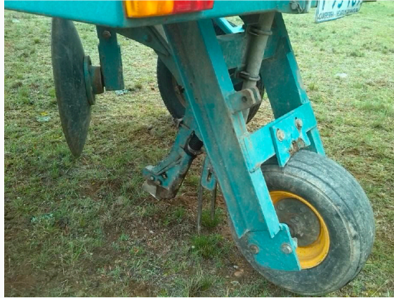
The Burford Seeder for the direct seeding of trees and shrubs
